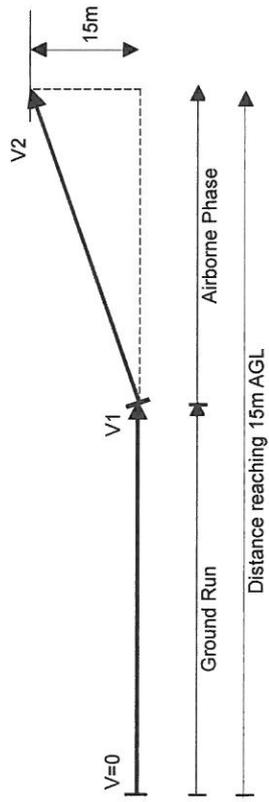
Normal Take Off over 15 Meter Obstacle and Ground-Run
