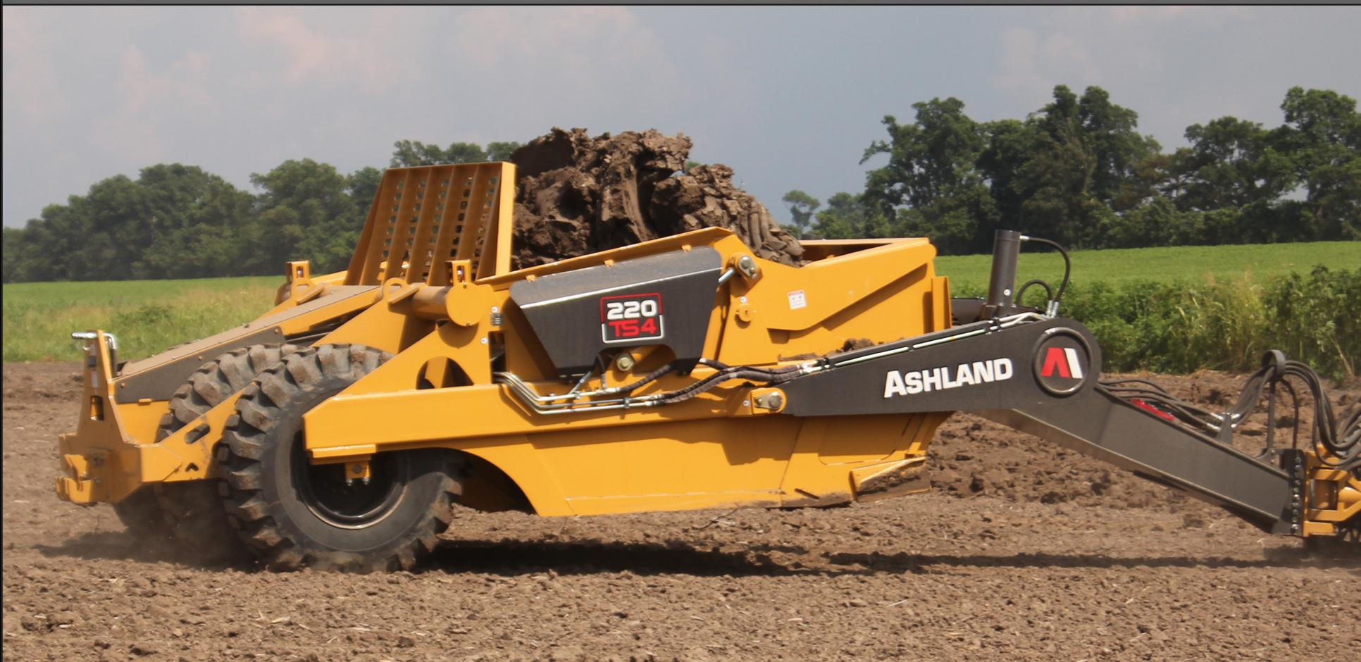
There is no such thing as too much strength. Friction welded cylinder rod eyes, a skeletal built Pole frame, heavy wall Front Section pipe, high grade steel – why sacrifice quality when you can upgrade to Ashland durability?
