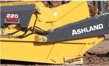
Our trunnion style lift cylinders attach the Bowl to the Front Section. They incorporate steel bands machined from a solid billet, heavy end caps, and through-grease trunnion mount blocks add up for more heft and convenient maintainance.
