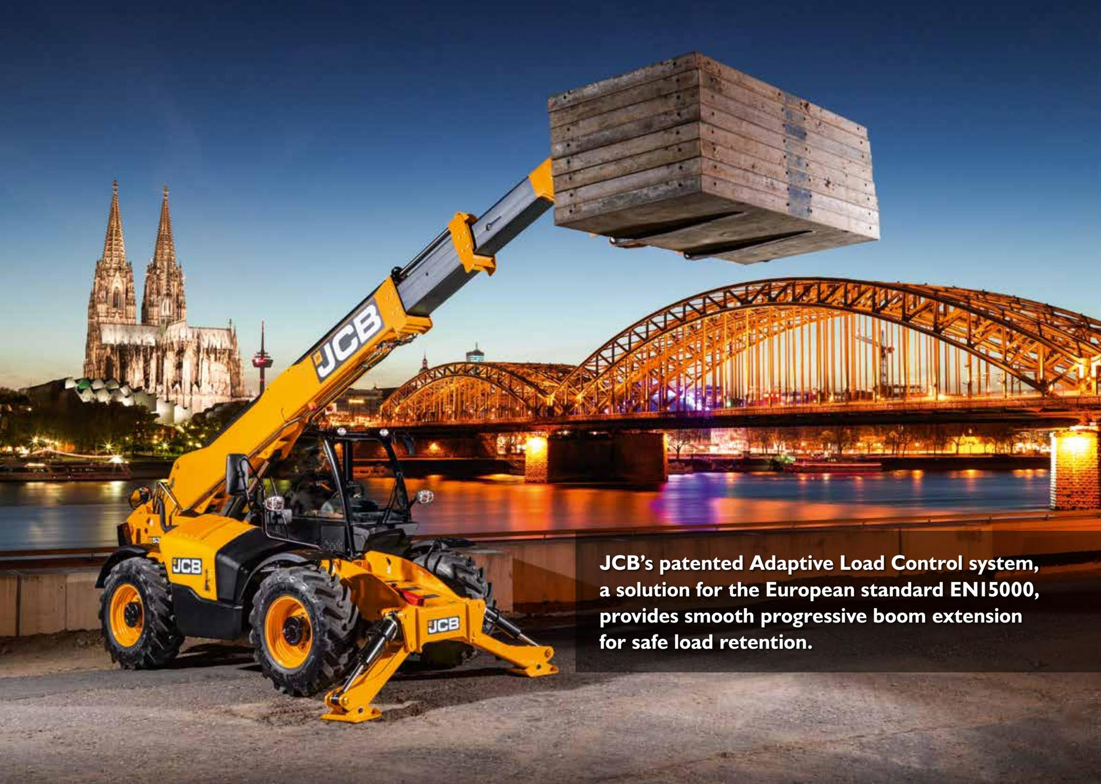
**JCB's patented Adaptive Load Control system, a solution for the European standard EN15000, provides smooth progressive boom extension for safe load retention.**
