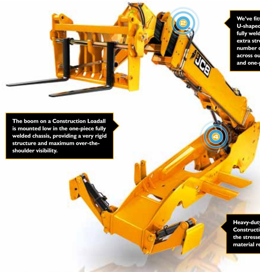
We've fitted a tough inverted U-shaped boom pressing with fully welded closing plates. For extra strength, we've reduced the number of joints and stress points across our integrated boom nose and one-piece closing plate.
