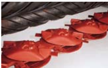
Two heavy-duty knives on each disc spin at 3,000 rpm for fast cutting without plugging.
