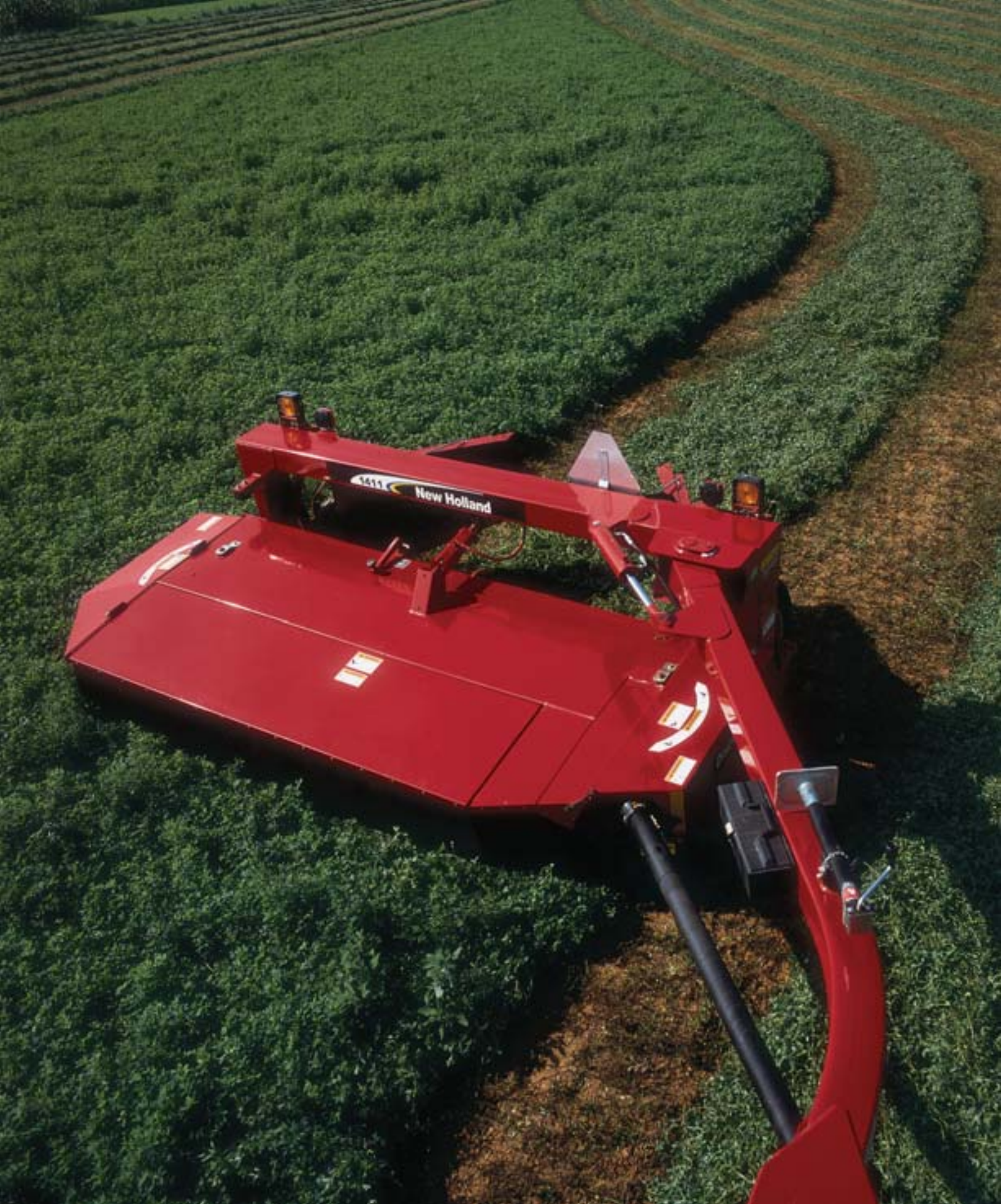
The Discbine header is suspended independently of the trail frame, allowing it to react both vertically and laterally to changing ground contours.
